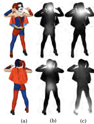
Fig. 3. Illustration of 6 partial point clouds, each line represents: (a) the rendered view, (b) the ground-truth saliency information and (c) the resulted saliency based on interpolation technique.
