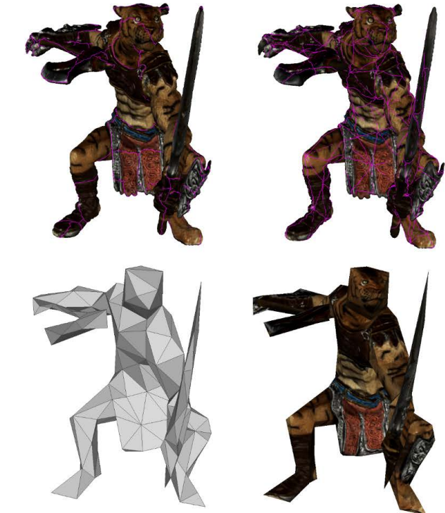
Figure 5: Re-atlasing. Top: input atlas and new atlas. Middle: input seams and seams after re-atlasing via the abstraction mesh. Bottom: abstraction and textured abstraction mesh.
