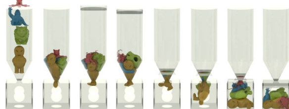
Fig. 1. Squeeze out: Incremental Potential Contact (IPC) enables high-rate time stepping, here with \Delta t = 0.01s , of extreme nonlinear elastodynamics with contact that is intersection- and inversion free at all time steps, irrespective of the degree of compression and contact. Here a plate compresses and then forces a collection of complex soft elastic FE models (B3K tetrahedra in total, with a neo-Hookean material) through a thin, codimensional obstacle tube. The models are then compressed entirely together forming a tight mesh to fit through the gap and then once through they cleanly separate into a stable pile.
