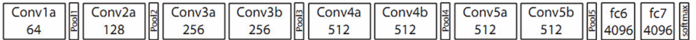
Fig. 2. The architecture of the C3D model (from Tran et al. 's paper [18]). It consists of 8 convolution layers, 5 pooling layers, 2 fully-connected layers and a softmax loss layer. The feature we extract is from fc6 layer, i.e., the first fully-connected layer.
