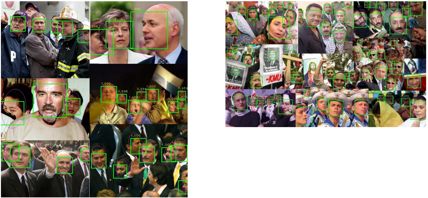
Figure 5: Examples of face detection in the FDDB dataset. The system is able to detect out-of-focus and occluded cases.
