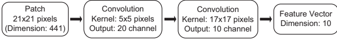
Fig. 3. The CNNs consist of two layers for encoding the local pattern. The input patch is 21 \times 21 in this paper, and the dimension of the output feature vector is ten.
