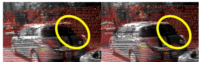
Fig. 1. Example of maximised MI. The projection of LiDAR points before (left) and after (right) the adjustment of extrinsic parameters is colour-coded by their intensity readings. The optimisation wrongly associates occluded points behind the car's back window.
