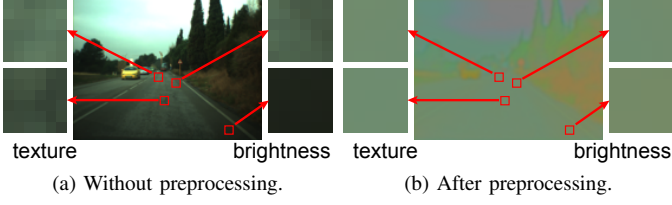
Fig. 2: A comparison on brightness and texture among different road areas (a) without and (b) after preprocessing.
