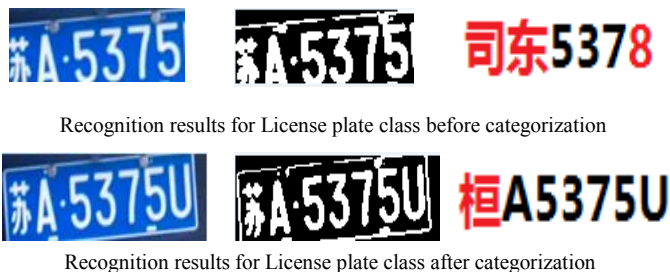
Fig. 2: Recognition results for the detected text lines corresponding to text detection before and after classification. Note: errors are indicated in red.
