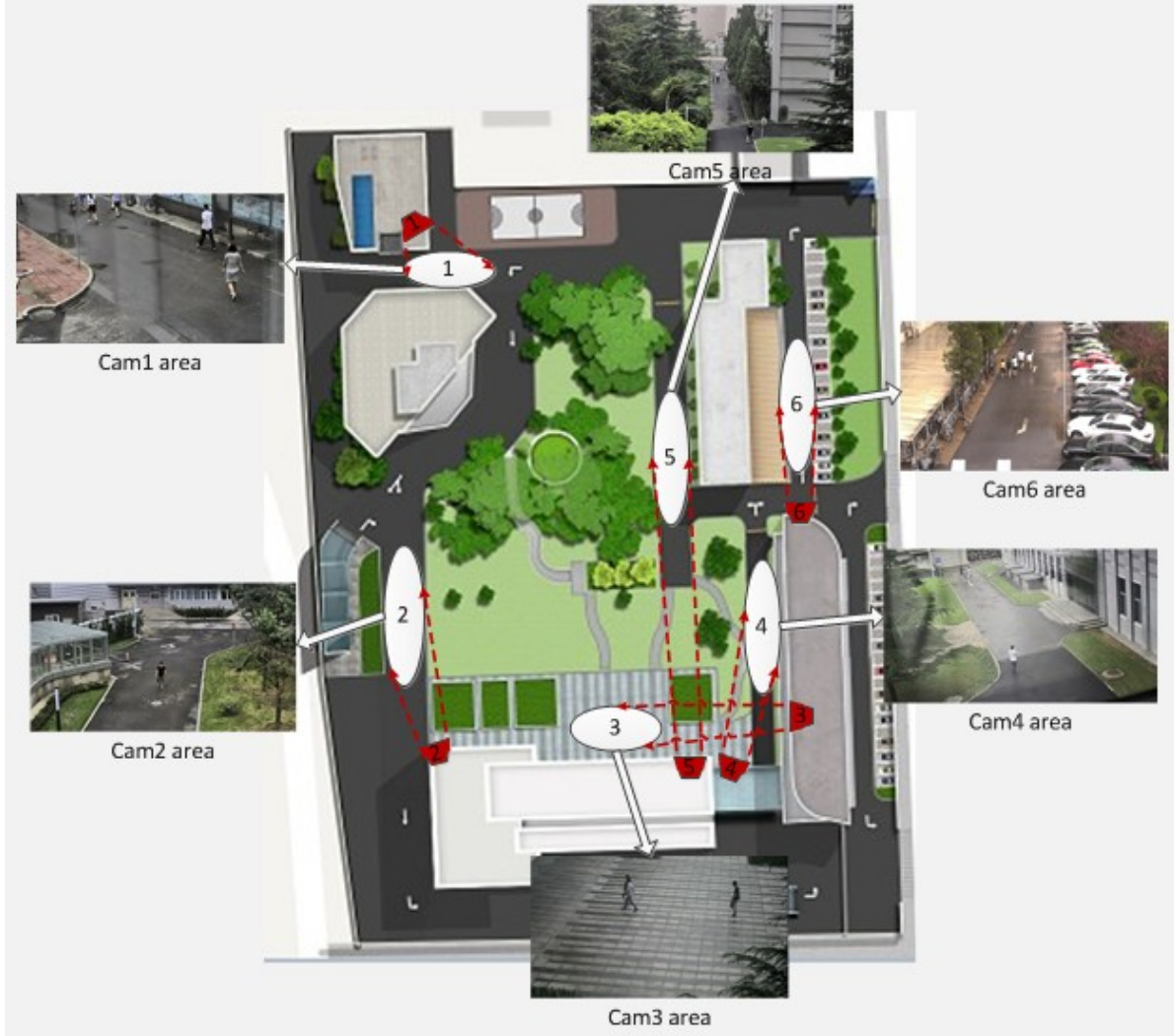
Fig. 1. The layout of the site. The white ellipse areas indicate the FOV of a single camera, and the arrow points to the corresponding actual scenario. The red trapezoid blocks denote the positions where we locate the cameras. Best viewed in color.
