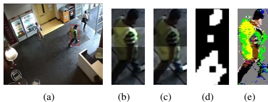
Fig. 3. An image to be searched, and a particle location (red bounding box) are shown in (a). Given this particle location, regions of interest for the torso (b) and legs (c) are defined. Within each of these regions, the motion (d) and colour (e) are considered and used to determine how well the candidate bounding box matches the query (note that when considering the colour, a soft decision approach is used rather than the hard decision indicated by (e)).
