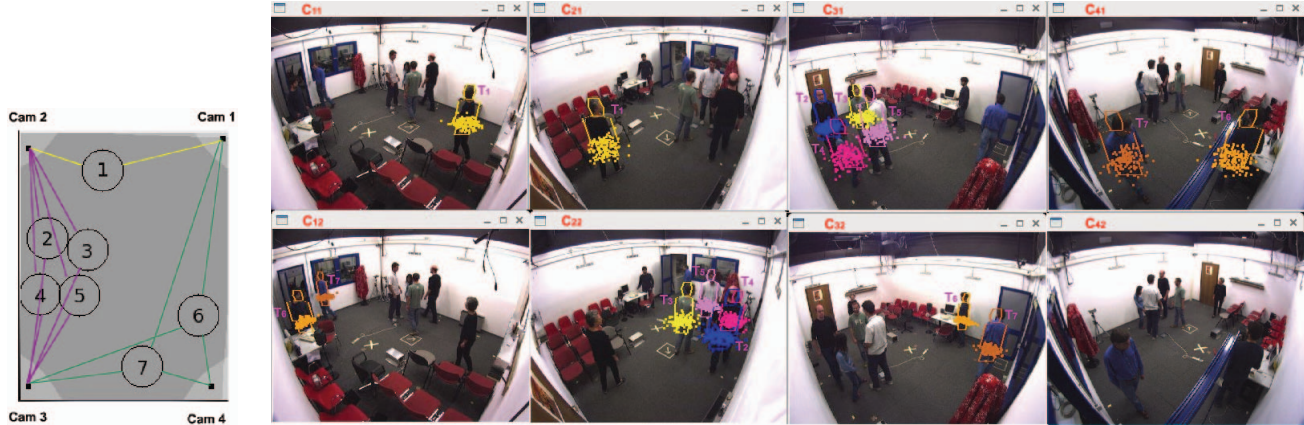
Fig. 5: A screenshot of the tracker. The left is the map. On the right there are 8 camera views, with the second row being a copy of the first row (i.e., C_{12} and C_{11} both refer to Cam 1.). The lines connecting a target to cameras indicate the target is tracked by the corresponding cameras. The dots around the targets are particles (hypotheses).
