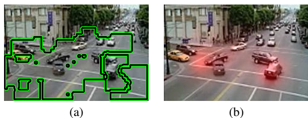
Fig. 6. The accident localization of each algorithm (a) Intelligent Driver Model (b) Proposed Method. Best viewed in color.
