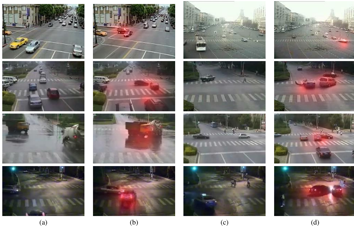
Fig. 5. The detection result of car accident dataset. Column (a) and (c) are the sample frames in normal situation of each video. Column (b) and (d) are the detection results of proposed method when traffic accidents occur. Best viewed in color.
