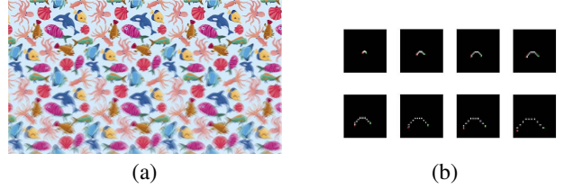
Fig. 2. (a) Motion blurred planar scene. (b) PSFs at different locations of (a).
