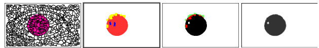
Fig. 4. From left to right: circle detected by circle fitting (purple) superimposed on the watershed transform, watershed regions totally overlapping the circle (red and blue) and partially overlapping the circle (yellow), result after the assignment to the foreground (black) of totally overlapping regions, subdivision of the partially overlapping regions.
