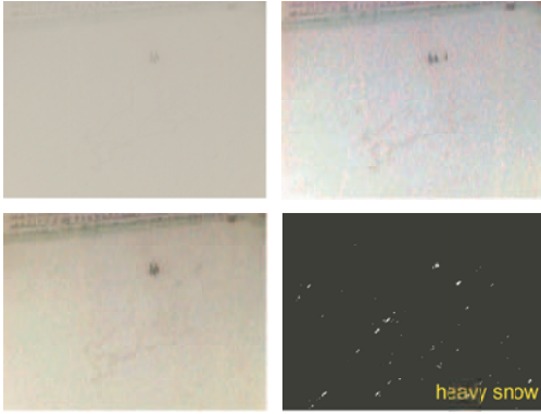
Fig. 6. The result of heavy snowfall. Top left: Input image; Top right: Fog removal image obtained by He et al. [10]; Bottom left: Fog removal image obtained by the proposed method; Bottom right: The result of snowfall detection
