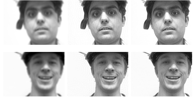
Fig. 5. Image deblurring comparison. (left)=Blurred images (middle)=deblurred with blind image deconvolution (right)=deblurred with aPCA-DWT.
