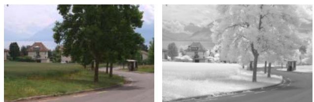
Fig. 1. Illustration shows intensity changes between RGB (left) and NIR (right) images when the same scene is acquired using RGB and NIR filters [1].
