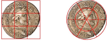
Fig. 8: Left: grid sub-regions. Right: the polar coordinate system. We build a histogram on each region and concatenate all the histograms to represent one image.
