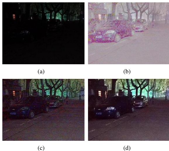
Figure 4. From top-left to bottom-right: input very low light level image, results by Multi-Scale Retinex in [2], method based on dark channel prior in [3] and the proposed method respectively.
