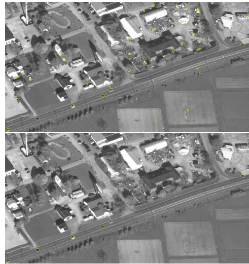
Figure 1: Moving vehicle detection results. Top: without scene context. Bottom: using context
