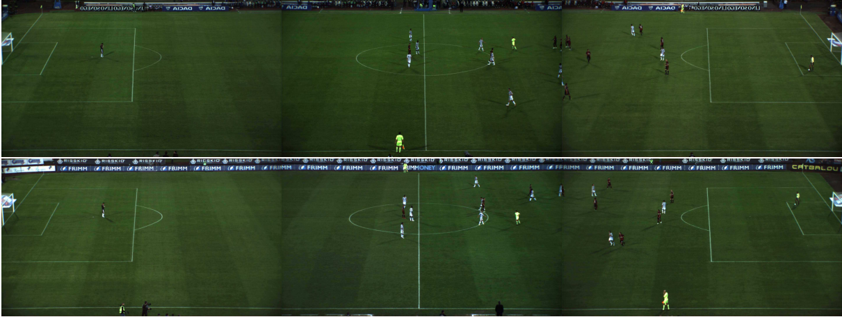
Figure 2. The global view of the field provided by the system at time t joining the images acquired from the six cameras placed in the stadium. We will call the three cameras on one side C6, C4 and C2, and the three cameras on the other side C5, C3, and C1 (from the left to the right, from the top to the bottom the corresponding images).
