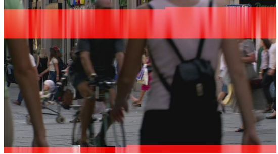
Figure 1 Original transmission error (error areas are tagged in red) Pedestrian Area sequence (TUM/Taurus Media Technik)
