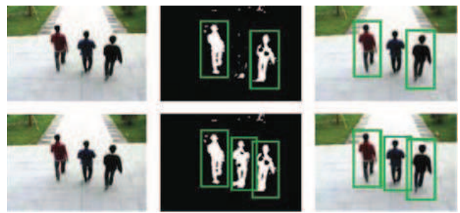
Fig. 4. The comparison between GMM and EGMM algorithms as filters for moving pedestrian detection. Top: GMM is used; Bottom: EGMM is used. EGMM can filter out all people (including still people from moving state), but GMM can not (such as the middle pedestrian of the picture). The binary result is through morphology dilate for a better view.
