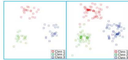
Fig. 4. (Left) scatter plot of 2D feature vectors and (Right) Resulting set of feature vectors after increasing the number of samples with rejection sampling [12].
