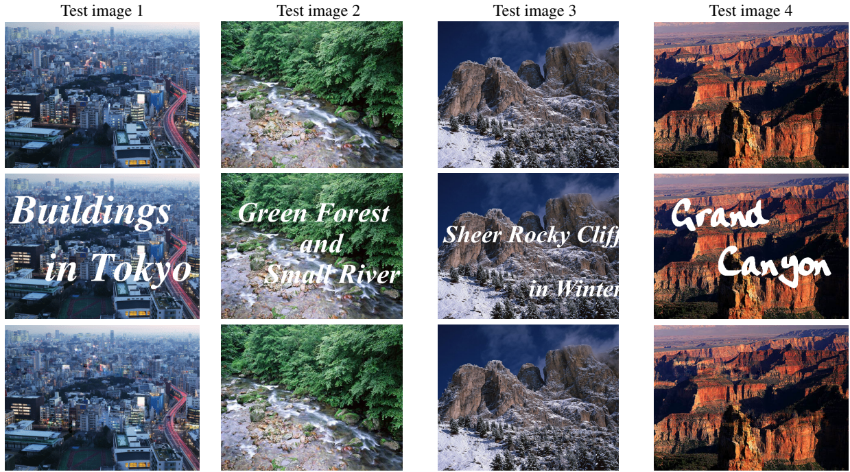
Fig. 3. Inpainting results obtained by the proposed method. Four test images are used, and the top, center and bottom rows are original images, corrupted images and inpainting results by our method, respectively. The sizes of Test images 1–4 are 480 \times 360 pixels, 640 \times 480 pixels, 640 \times 480 pixels and 480 \times 360 pixels, respectively. The percentages of missing areas are 10.7 %, 7.1%, 5.4% and 8.9 %, respectively.
