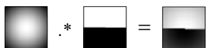
Fig. 1. Building a polarized Gaussian kernel by multiplying a Gaussian kernel with a binary mask, where ‘‘*’’ represents the element-wise multiplication.
