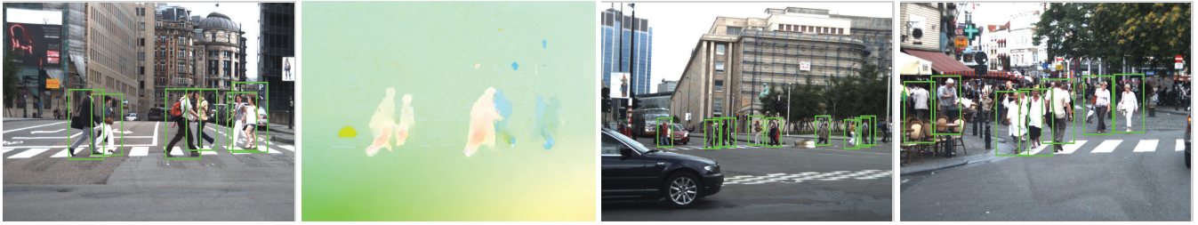
Fig. 3. Examples of pedestrian detections by HOG+CoF features. Detected bounding boxes are shown in green. The second picture shows colour coded optic flow map for the frame shown in the left.
