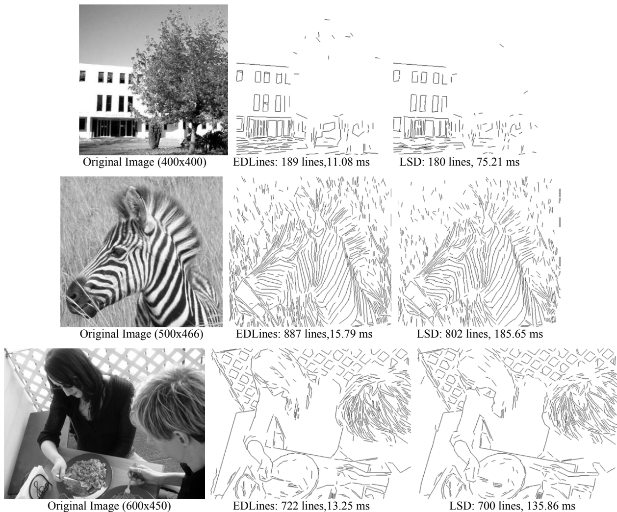
Figure 3: A comparison of EDLines to LSD on three challenging images. EDLines is 10 times or more faster than LSD while producing similar or better line segments. Both algorithms are run on a PC with an Intel 2.2 GHz CPU and 2 GB RAM.
