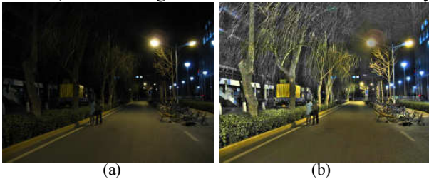
Figure 3 Enhanced image by SSR. (a) Input image. (b) Enhanced image after removing illumination.
