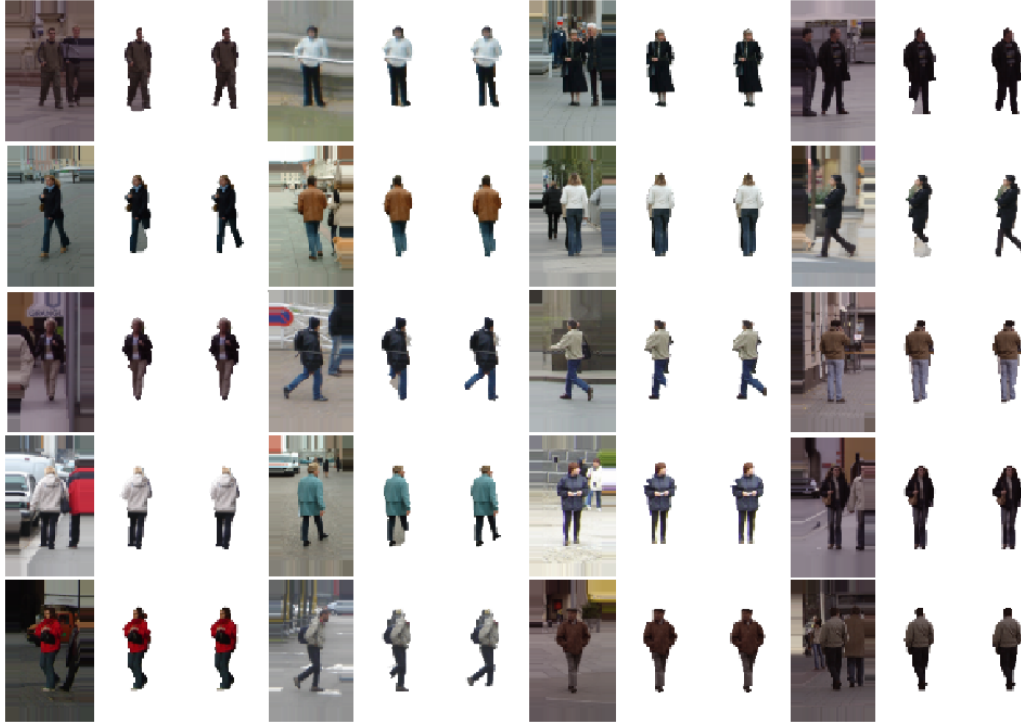
Fig. 5. From left to right: initial image, segmentation obtained with a single template and with a part-based template. In most of the cases, the segmentation is more accurate with the part-based template
