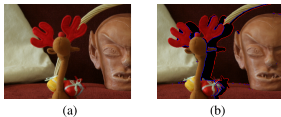
Fig. 3. Occlusion boundary labeling result. (a) Original color image. (b) Warped color image with occlusion boundary label (blue = foreground boundary, red = background boundary).
