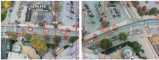
Fig. 1. A two camera view of a highway (traffic video surveillance). Moving vehicles are visible as red bounding boxes; the vertical lines mark the camera overlapping region.
