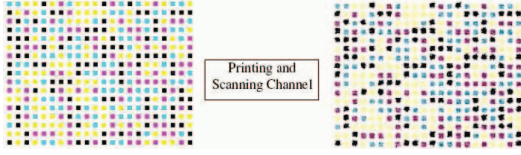
Fig. 2: Distortions in the PS channel.
