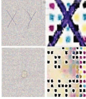
Fig. 3: External distortions due to pen scribing and coffee spills.
