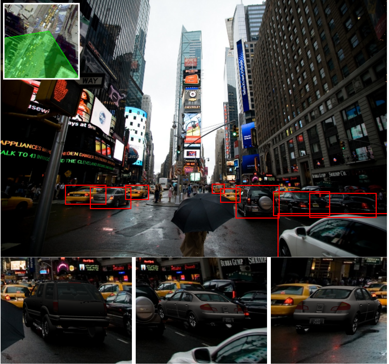
Figure 3. Example 1. A wide-angle daytime photograph. The photograph is annotated with bounding boxes around each labeled vehicle, and several 3D ground truth labeled car poses are shown underneath. The estimated pose of the camera is shown in the overlay at the top left. Note that even with a large degree of perspective distortion, the labeler was able to accurately annotate the photograph, because we use the recovered camera intrinsics in the 3D annotation tool.
