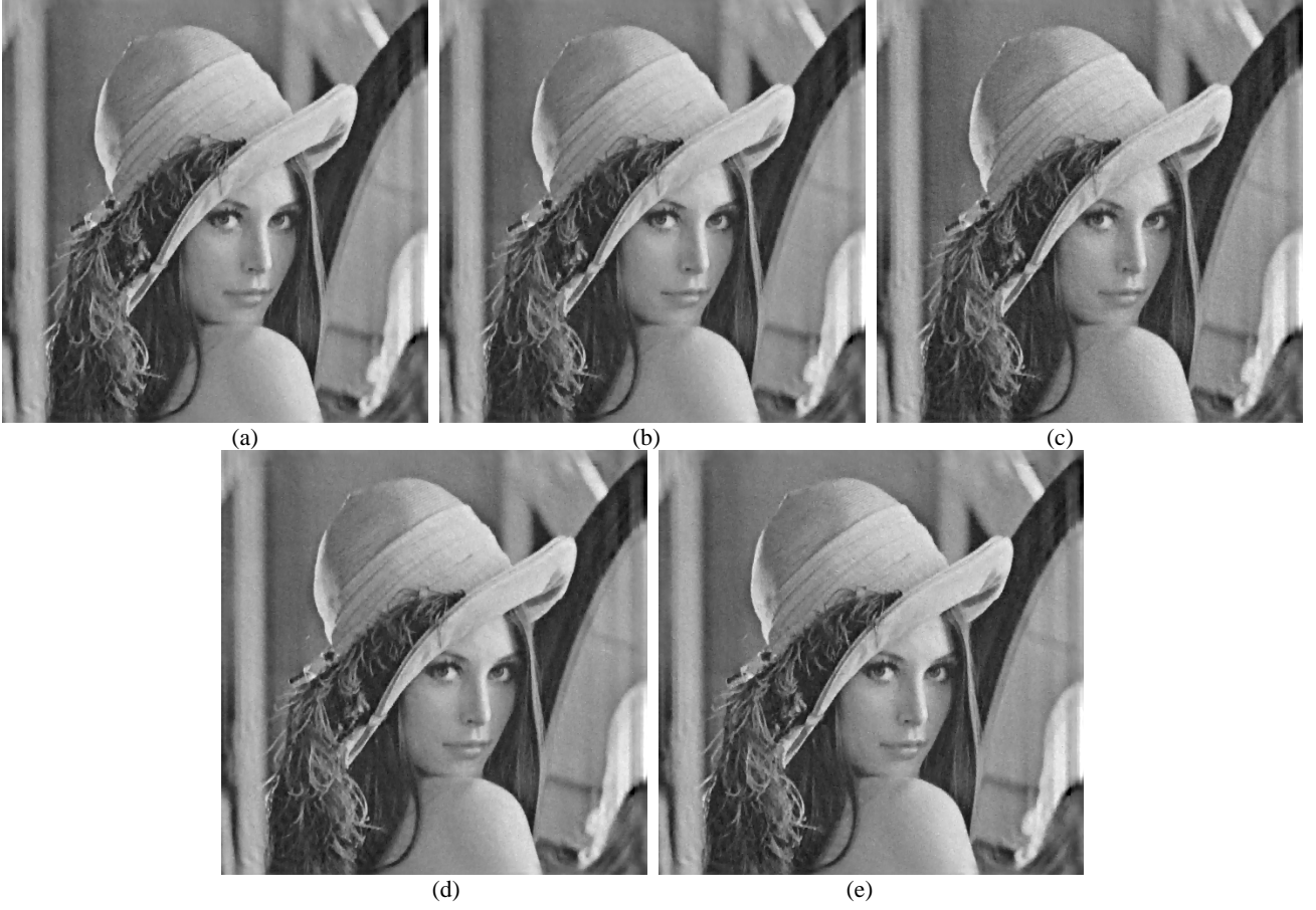
Figure S-6. Deconvolution results on images (im1) blurred by kernel5 by using: (a) GISA, (b) LUT, (c) IRLS, (d) IRL1, and (e) ITM- l_p .
