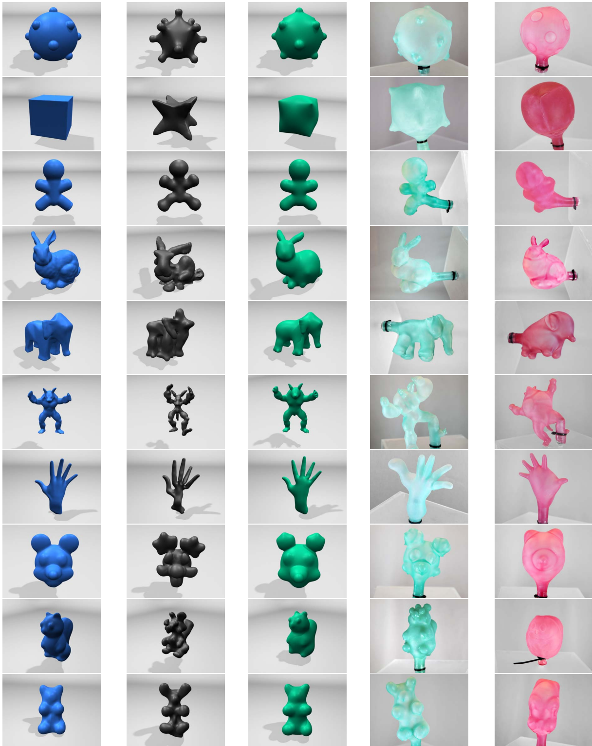
Figure 4: Results obtained with our method. The columns (from left to right) show target shapes, optimized balloons, simulated inflated balloons, fabricated optimized balloons and fabricated balloons corresponding to downscaled targets.
