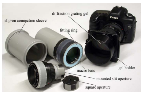
Figure 4: The disassembled objective showing the imaging lens (left). The collimating lens is mounted inside the PVC tube with the slip-on pipe connection sleeve (middle). The gel holder containing the diffraction grating is directly mounted to the re-imaging lens on the camera (right).
