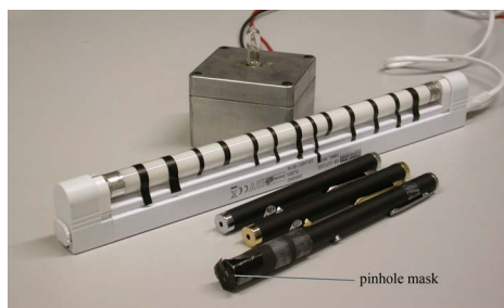
Figure 5: The calibration equipment consisting of a calibration halogen lamp (top), a striped fluorescent lamp (middle) and red, green and blue laser pointers and a pinhole mask (bottom).
