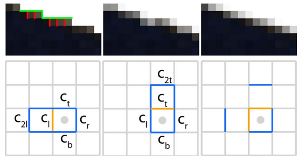
Figure 5: Top: Dominant contrast in green edges should mask the spurious red crossing edges (left). Not taking this local contrast into account leads to artifacts (center). Our SMAA algorithm corrects them (right). Bottom-left: left boundary (orange) of a given pixel (marked with a dot) and surrounding candidate edges (blue) that may dominate it, making it non-visible for human viewers. Bottom-middle: top boundary scenario. Bottom-right: candidate surrounding edges actually calculated.
