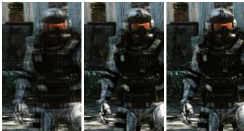
Figure 12: Left: Using a naive resolve results in visible ghosting. Middle: Reprojection mitigates these artifacts but does not completely remove them. Right: The addition of velocity weighting allows to completely remove ghosting.
