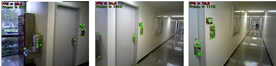
Fig. 4. FAST corners and their correspondences from the last key-frame after refinement.
