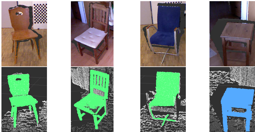
Fig. 2. The top row shows example objects from our evaluation. Chairs and stools served for the two fine-grained affordances. The bottom row presents affordance detection results: the sitting with backrest affordance is shown in green, whereas the sitting without backrest affordance is shown in blue.
