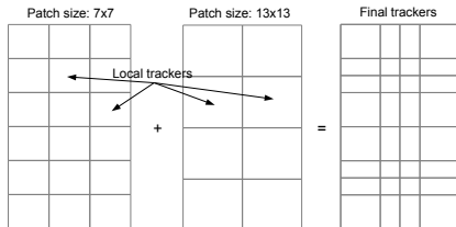
Fig. 3. The final trackers are obtained by superimposing grids with different patch sizes. In this case two grids with a size of 7x7 and 13x13 pixel. Using patches with different sizes ensure a greater robustness over different appearances of objects.
