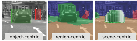
Fig. 1. Different scene representation levels trading-off specificity (object-centric) and generality (region-centric). We advocate the use of a medium-level scene-centric model to balance this trade-off and gain efficiency.
