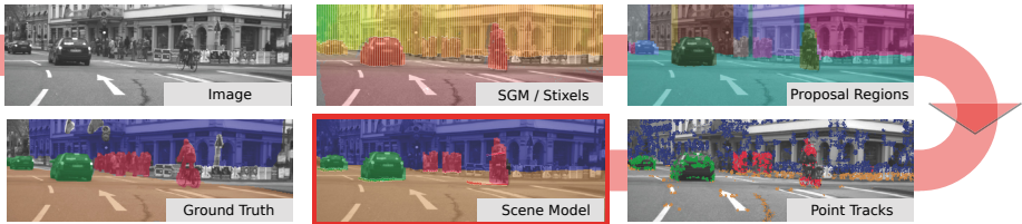
Fig. 2. System overview. A spatio-temporally regularized medium-level scene model (bottom center) is estimated in real-time. This model represents the scene in terms of 3D scene structure, 3D velocity and semantic class labels at each Stixel. Dense stereo and Stixel visualization (top center) is color-encoded depending on distance. Stixel-based proposal regions for classification are shown in false-color (top right). In all other images, colors represent semantic object classes.
