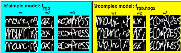
Fig. 5. Here, we examine the histogram at .62 budget from Fig. 4c. We provide examples of three different words being classified at the cheapest/simplest model ( f_{rgb} ) and at the complex/expensive model ( f_{rgb,hog2} ). As expected, more obscure and rotated words require the complex model.
