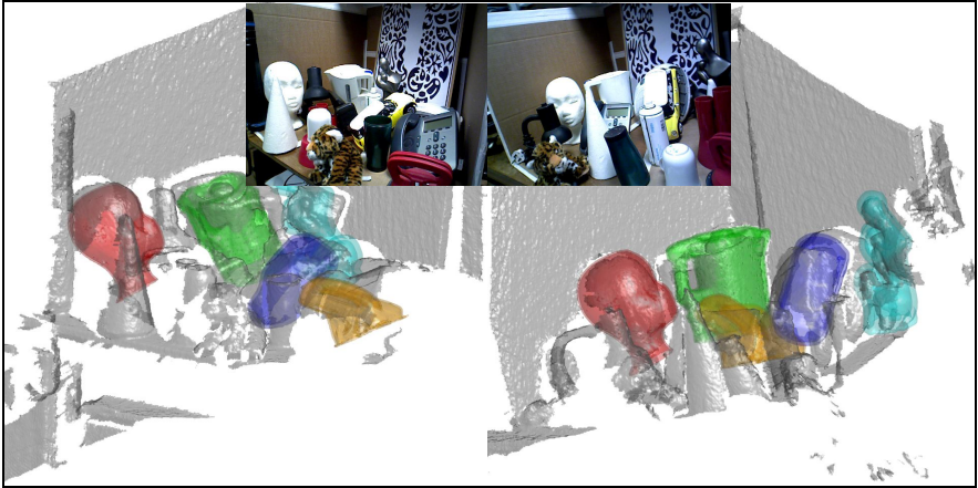
Fig. 1. Sample results of our instance recognition method which uses only point clouds as input. Meshed scenes from our Desk3D dataset with results of detection and pose classification on five object instances. Note meshed scenes are shown only for better visualization. Best viewed in color. See supplementary for videos.
