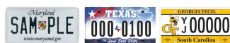
Fig. 2. License plate templates showing typical difficulties for ALPR systems: state symbols, stacked characters, complex backgrounds
