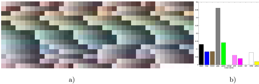
Fig. 11. Patches of the Munsell atlas considered statistically equivalent to an ideally white surface for von Kries adaptation under all the illuminants and sensor filter sets considered (a). Their color names histogram (b).
