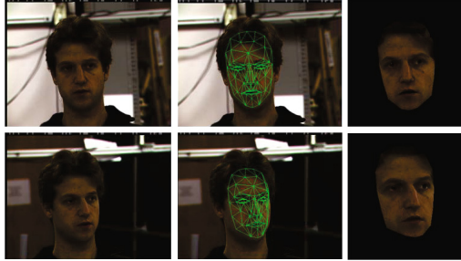
Fig. 3. Model fitting to two example images and texture projection on 3D surface after perspective correction. Images are taken from CMU-PIE database [21].
