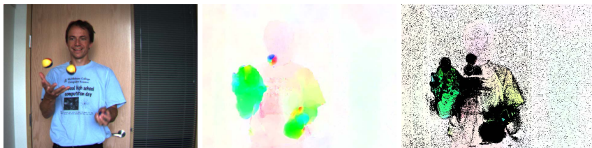
(a) First input frame (b) Dense flow estimation (c) Reliable flow estimates
