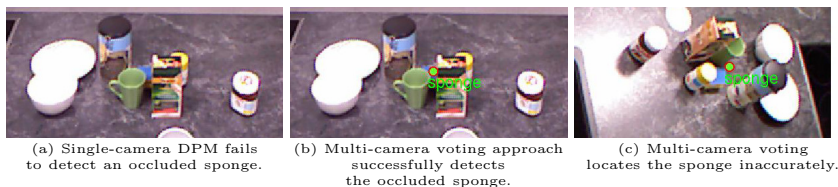
Fig. 5. Multi-camera voting approach successfully detects an occluded object
